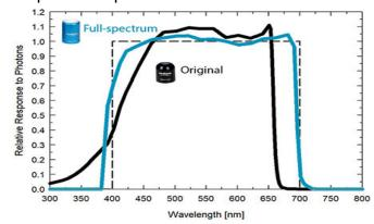
Mean **spectral response** measurements of six replicate Apogee MQ-210 and MQ-510 series quantum sensors. Spectral response measurements were made at 10 nm increments across a wavelength range of 300 to 800 nm in a monochromator with an attached electric light source. Measured spectral data from each quantum sensor were normalized by the measured spectral response of the monochromator/electric light combination, which was measured with a spectroradiometer.
